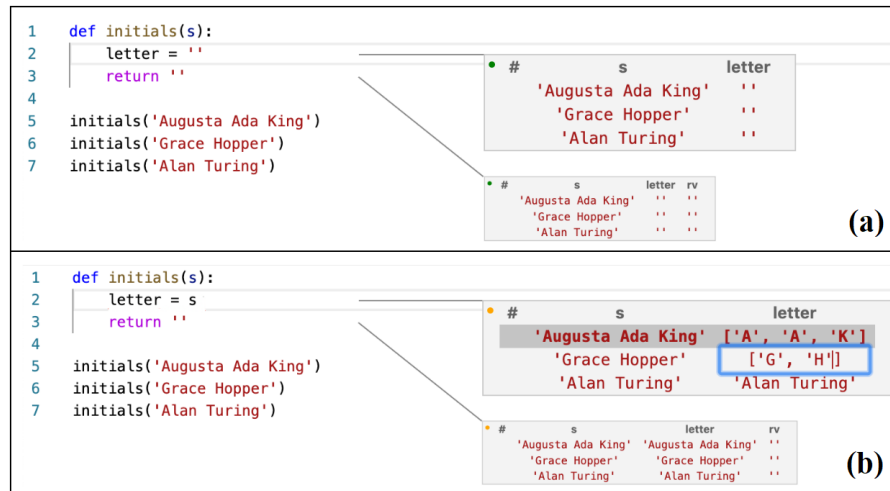
Figure 1. Program synthesis with SNIPPY: (a) the user observes values of variables in the Live Programming environment; (b) providing output values creates input-output examples to be passed along to synthesis. Figure originally from [8].
